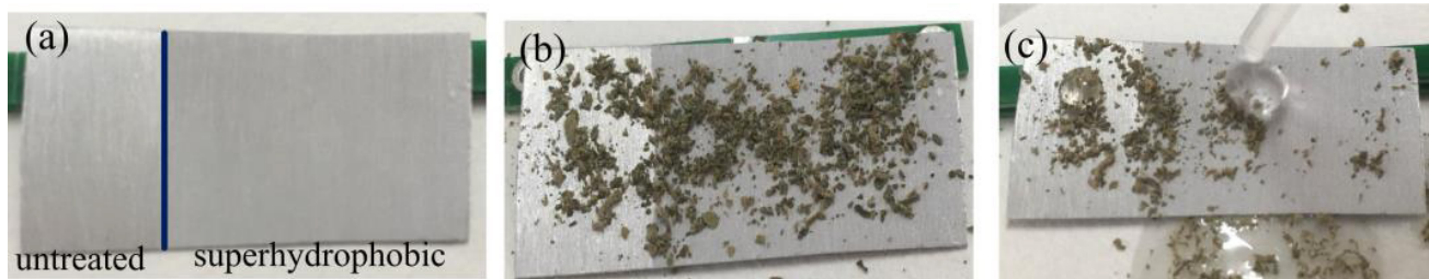
Figure 4 Self-cleaning property of the superhydrophobic surface.
