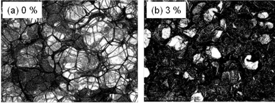
**Figure 2** SEM images of PEDOT:PSS thin films fabricated in the foam network analyzed by Image J program (a) without and (b) with 3 wt.% SDS surfactant. Opaque part represents the coated thin films, while transparent part is without films.
