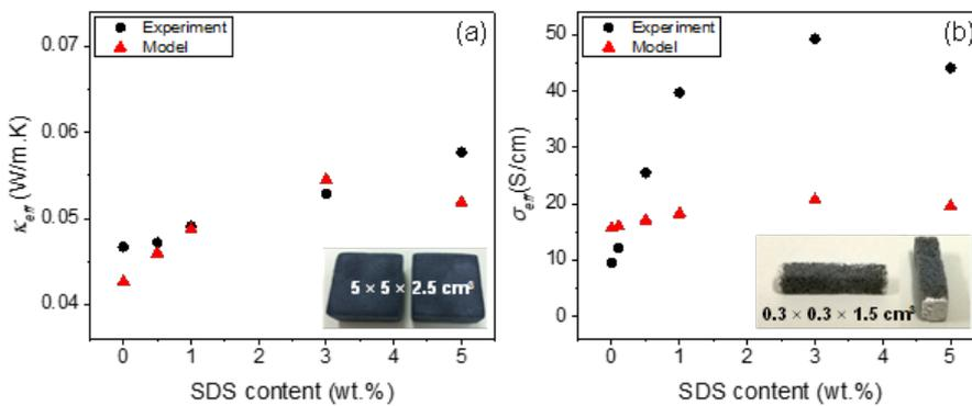
**Figure 3** Modeling and experimental results of (a)  $k_{eff}$  at  $t_k = 0.4$  (sample size:  $5 \times 5 \times 2.5 \text{ cm}^3$ ) and (b)  $\sigma_{eff}$  at  $t_\sigma = 0.015$  (sample size:  $0.3 \times 0.3 \times 1.5 \text{ cm}^3$ ).
