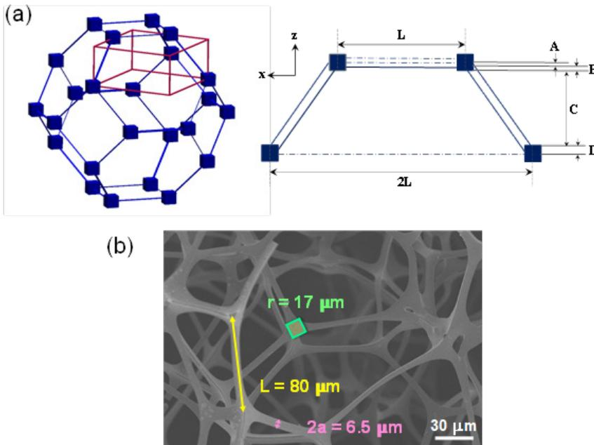
**Figure 1** (a) Schematic diagram of the layered hexahedral unit cell of Boomsma-Poulikakos's model and (b) SEM image of melamine foam network.
