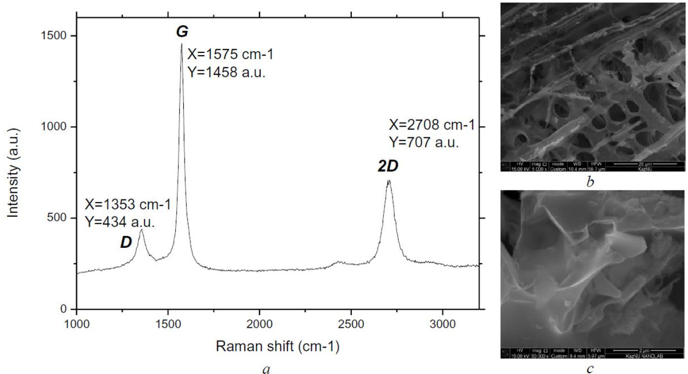
**Figure 1** (a) Raman spectrum of a multilayer graphene and SEM microimages of the graphene film on areas of (b)  $60 \mu\text{m} \times 50 \mu\text{m}$  and (c)  $6 \mu\text{m} \times 5 \mu\text{m}$ .
