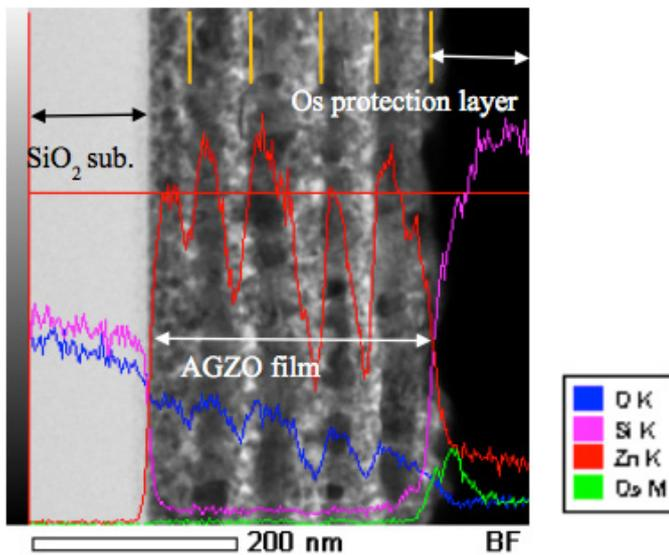
**Figure 4** Expanded cross-sectional TEM image of quintuple-layer AGZO film and corresponding EDS analysis. Five yellow lines are eye-guides to separate the stacked five layers. EDS analysis indicates four atom distributions: zinc (red), oxygen (blue), silicon (pink), and osmium (green). Sample was covered by Os protection layer. SiO<sub>2</sub> substrate was cleaned by SC-1 method.
