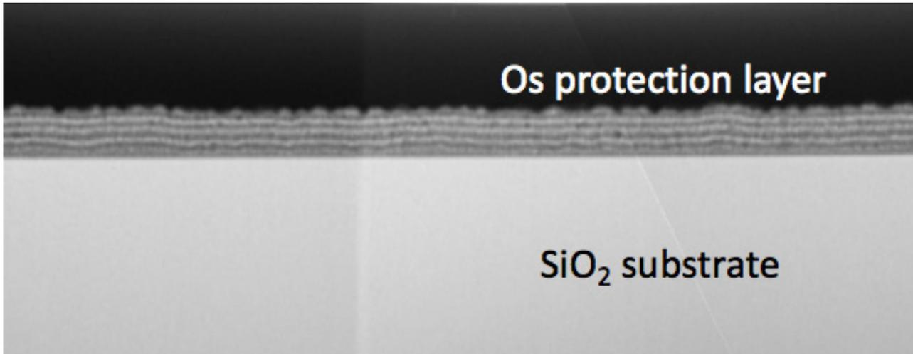
**Figure 3** Cross-sectional TEM image of quadruple-layer AGZO film. Five periods of bright and dark layers correspond to fabricated quadruple-layer AGZO film.
