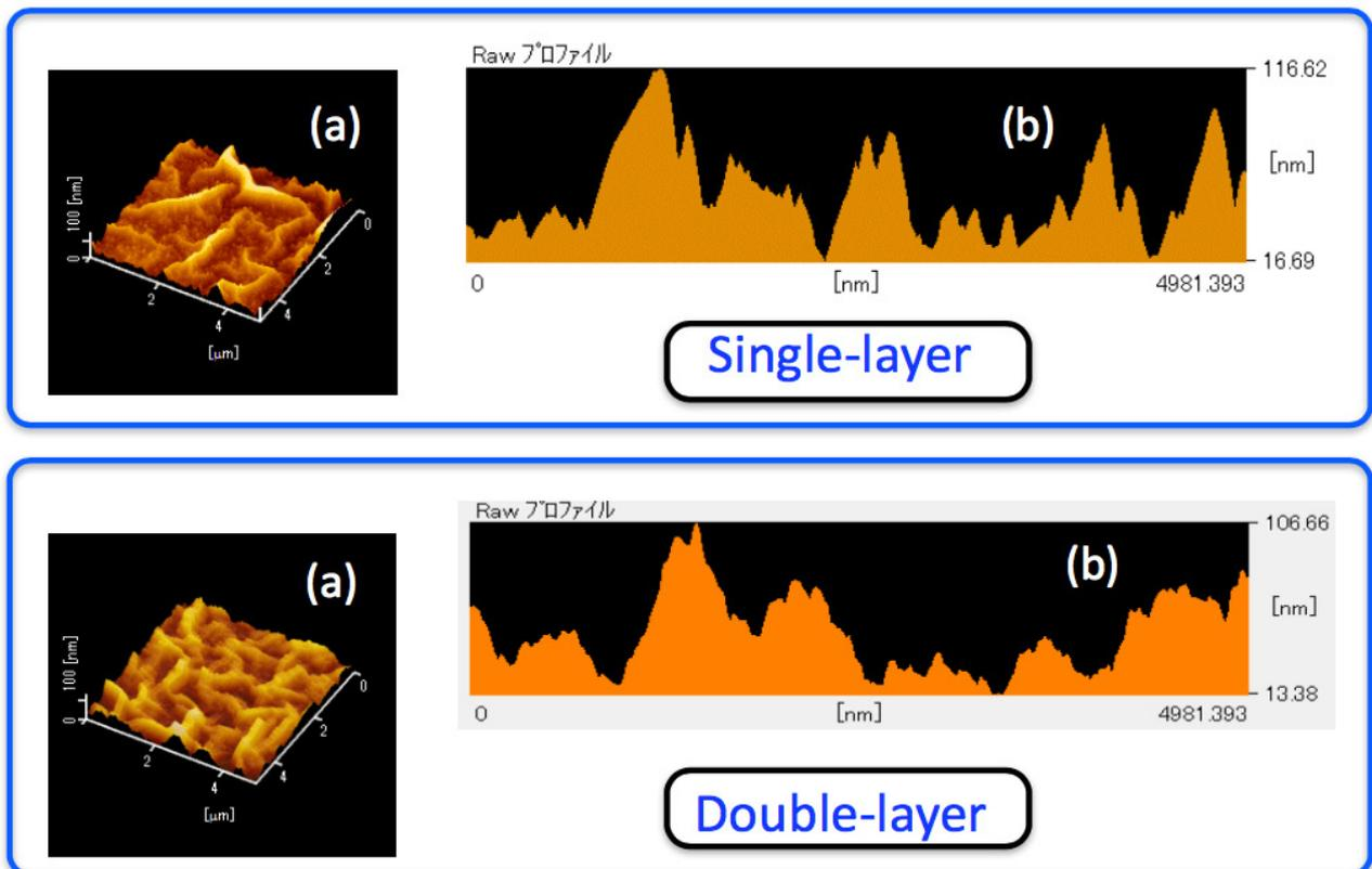
**Figure 1** AFM images of the single- and double-layer AGZO films: (a) their surfaces and (b) crosssectional images.
