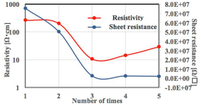
**Figure 2** Resistivity (red line) and sheet resistance (blue line) of samples from single- to quintuplelayer AGZO films fabricated on glass substrates cleaned using SC-1 method.
