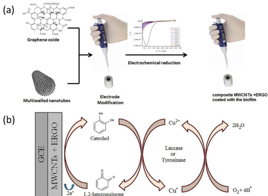
**Figure 1** Preparation steps of the biosensors based on Tyr or Lac (a) and schematic of the reactions occurring within the biofilm and at the interface with the modified GCE (b).
