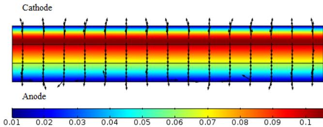
**Figure 2** Temperature distribution (K over 800C) and total heat flux vectors in the 2D simulation (cell potential 0.6V).
