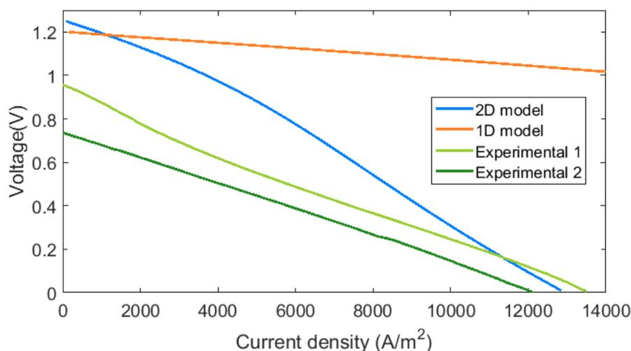
**Figure 3** Comparison of the modelled and experimental JV curves from 1D and 2D simulations and nanocomposite cell measurements.
