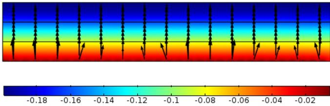
**Figure 1** Ionic potential distribution (V) and ionic current density vectors in the 2D simulation (cell potential 0.6V).
