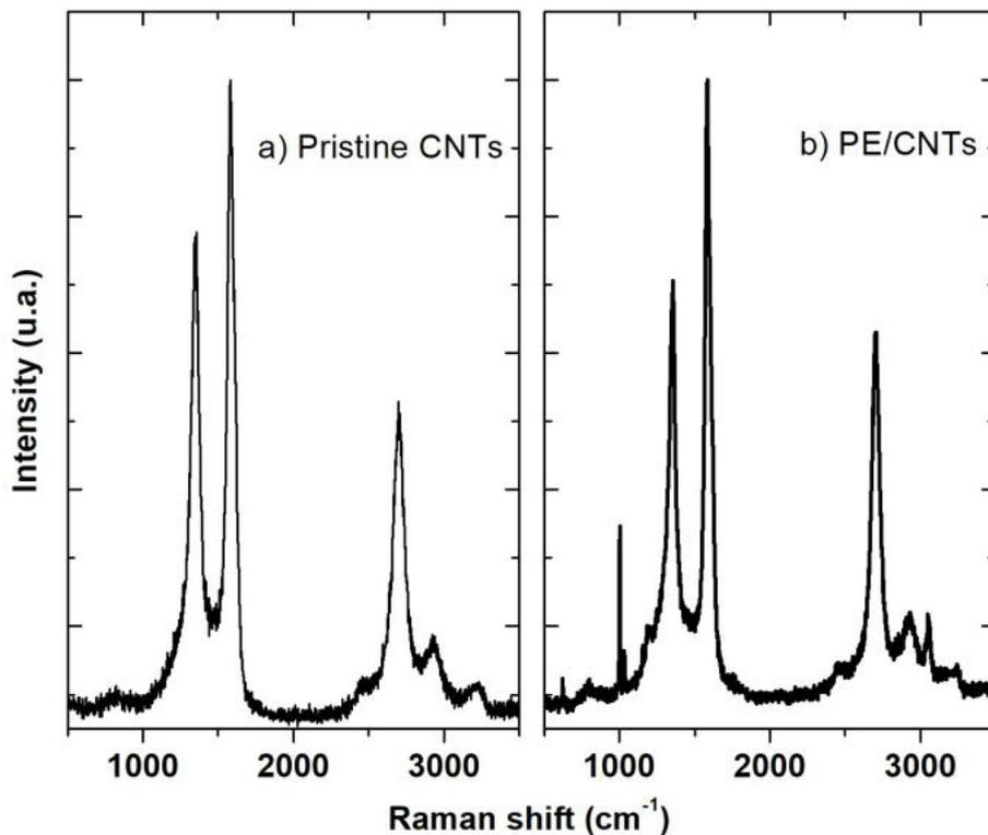
**Figure 2** Raman spectra of pristine CNTs (a) and polyethylene (PE) layer on super-hydrophobic CNTs/steel screen (b) with a 514 nm laser line.
