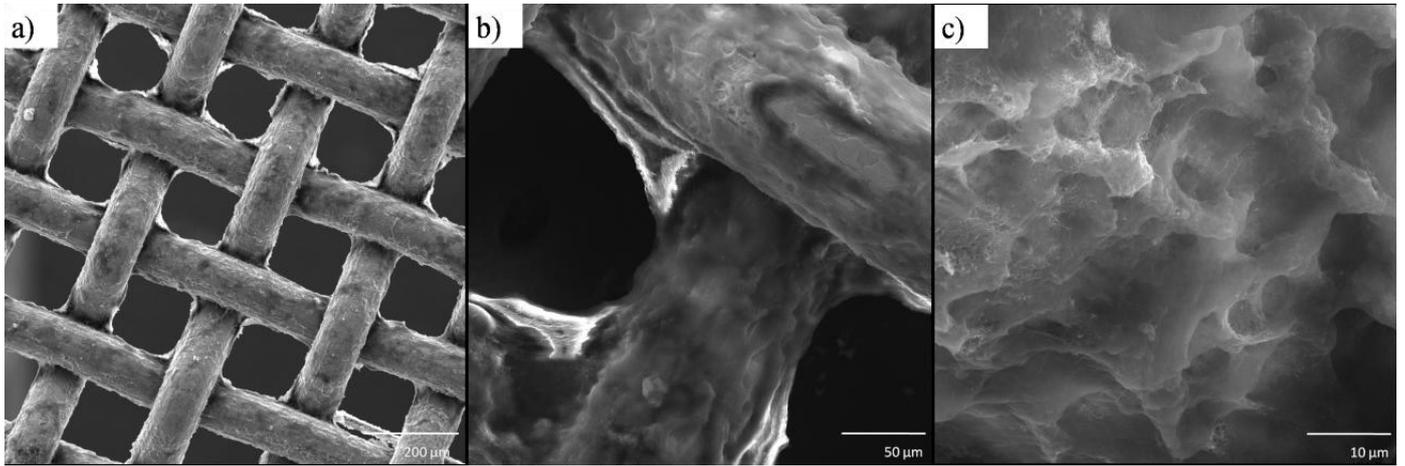
**Figure 1** SEM micrographs of polyethylene (PE) layer on super-hydrophobic CNTs/steel screen at 100x (a), 1kx (b) and 5kx (c).
