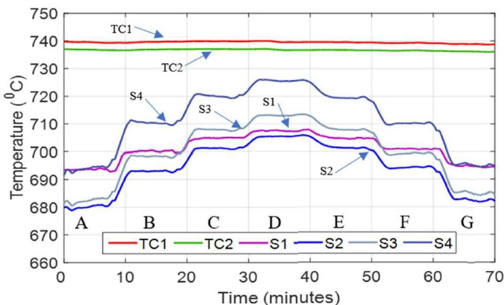
**Figure 1** Temperature response to varying flow rates.
