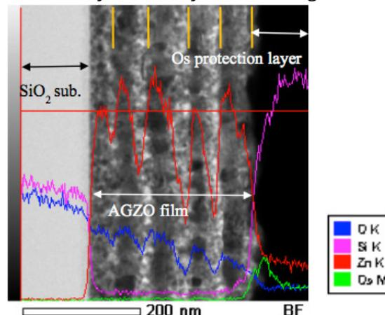
**Figure 2** Cross-sectional TEM-EDS image of quintuple-layer AGZO film, indicating four atom distributions: zinc (red), oxygen
