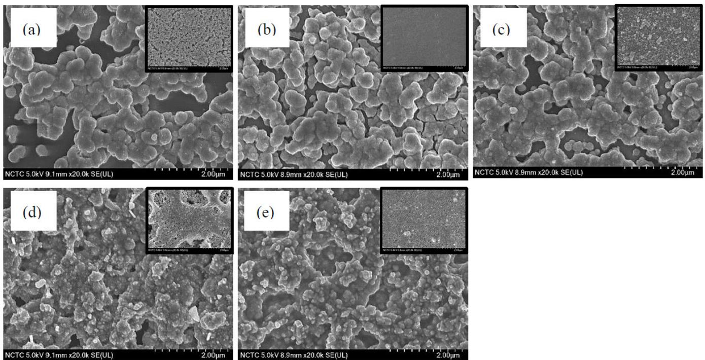
**Figure 1** (SEM micrographs of CZTS thin films prepared at deposition speeds of (a) 500  $\mu\text{m/s}$ , (b) 750  $\mu\text{m/s}$ , (c) 1000  $\mu\text{m/s}$ , (d) 1250  $\mu\text{m/s}$ , and (e) 1500  $\mu\text{m/s}$ , annealed at 440°C. Insets show films prepared at corresponding deposition speeds and annealed at 340°C.
