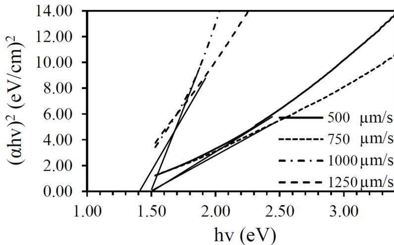
**Figure 3**  $(\alpha hv)^2$  vs.  $h\nu$  of CZTS films, prepared at various deposition speeds annealed at 340°C.
