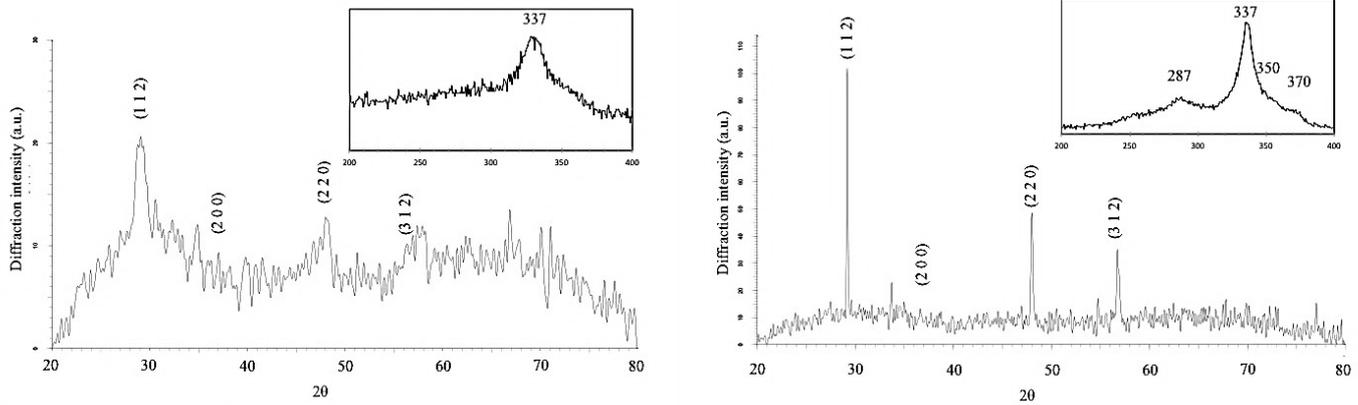
**Figure 2** XRD spectra of CZTS thin films prepared at deposition speed of 750  $\mu\text{m/s}$  and annealed at a) 340°C and b) 440°C. Insets show Raman spectra of corresponding CZTS thin films.
