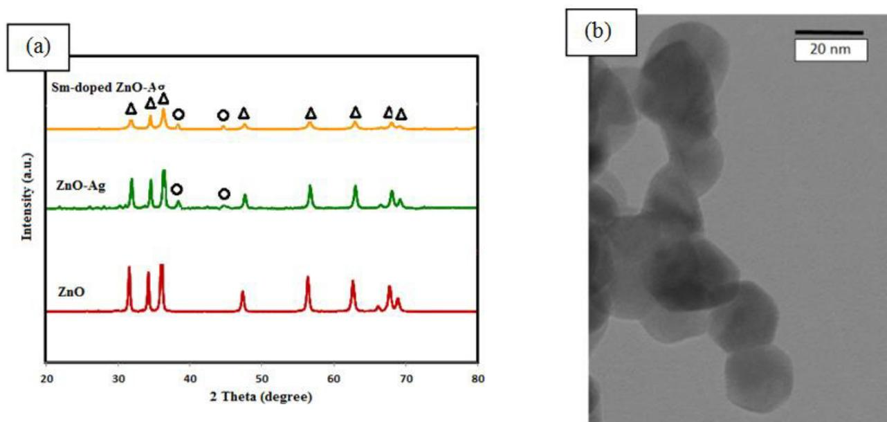
**Figure 1** (a) XRD patterns of pure ZnO, ZnO-Ag, and Sm-doped ZnO-Ag calcined at 500 °C and (b) TEM image of Sm-doped ZnO-Ag calcined at 500 °C.
