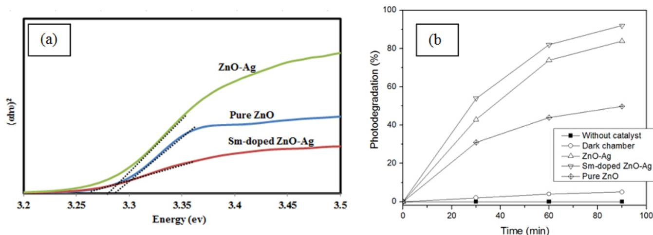
**Figure 2** (a) The plots of  $(\alpha h\nu)^2$  versus photon energy ( $h\nu$ ) and (b) photodegradation efficiency of pure ZnO, ZnO-Ag, and Sm-doped ZnO-Ag calcined at 500 °C.
