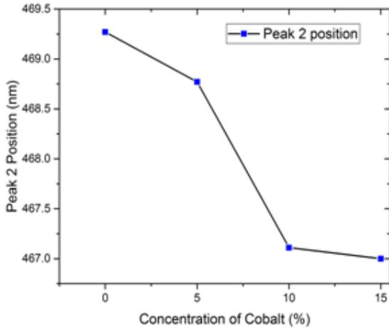
**Figure 7D** Position of Peak 2 of Quantum dots.
