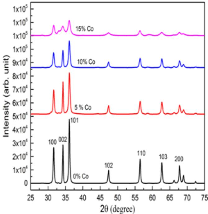
**Figure 3** Powder X-ray diffraction of QDs.
