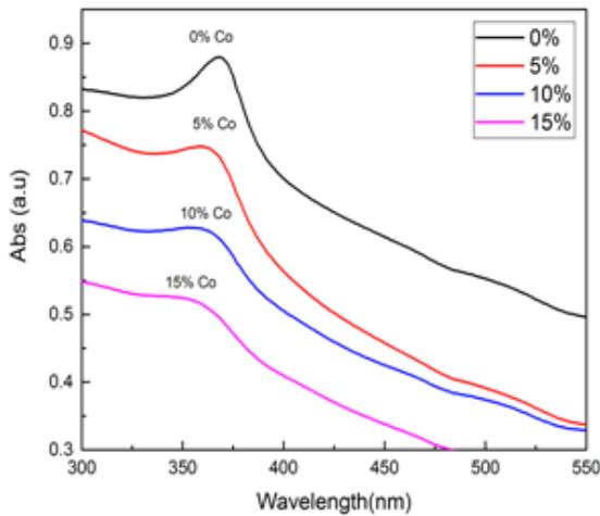
**Figure 5** Absorption Spectra of cobalt doped QDs.
