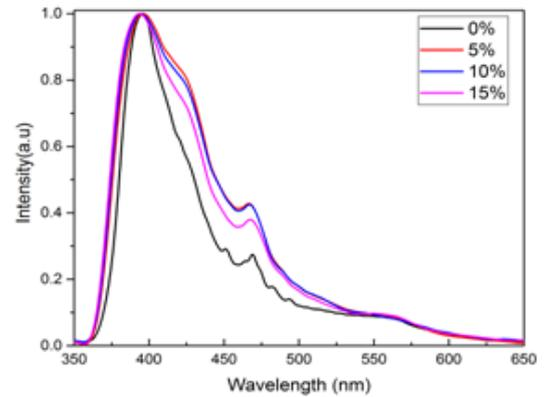
**Figure 7A** PL measurement of Quantum dots.
