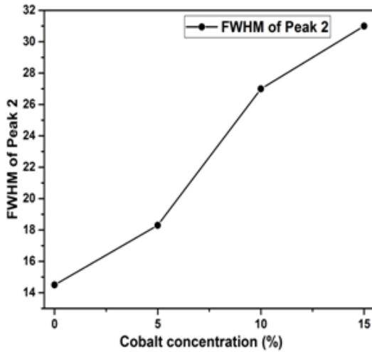
**Figure 7E** FWHM of Peak 2 of Quantum dots.
