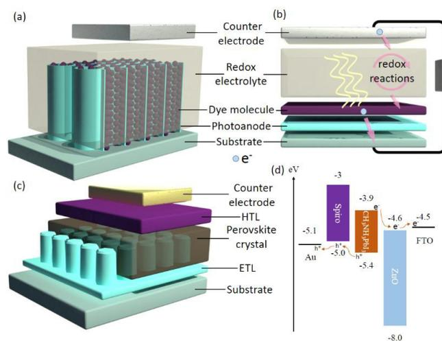
**Figure 1** (a) Schematic configuration of DSSC, (b) basic working principle of DSSC, (c) Schematic configuration of PSC, (d) basic working principle of PSC.
