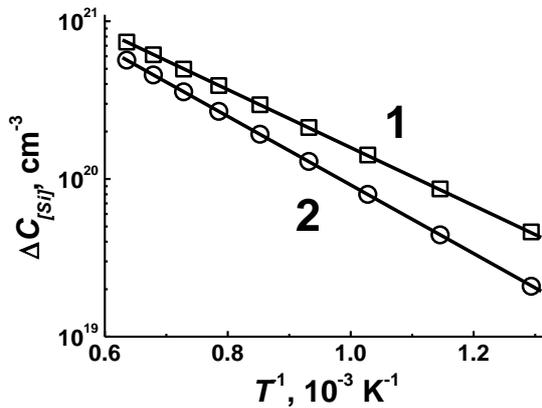
**FIGURE 2.5** Dependence of the solubility limit of Si in  $\text{SiO}_2$  phase on the inverse temperature for the a-Si / Si oxide (1) and the c-Si / Si oxide (2) systems. Symbols present the results of calculations by the expression
